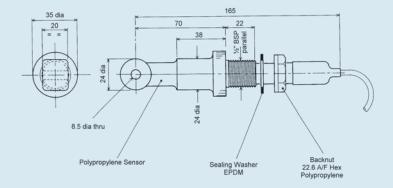
NOTE: 22.0 - 21.4 diameter hole required for fitting
