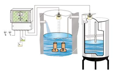
The Swing unit has been designed for either 1 or 2 sensor inputs & can provide 2 isolated 4-20mA outputs & 5 relay outputs.
